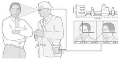
Above: Illustration of The Emotional Social Intelligence Prosthetic that vibrates whenever the listener's attention veers off topic. The eventual goal for the system is to provide the mildly autistic with an auxiliary notification of other people's emotions on a daily basis. (Source: Rana el Kaliouby)
