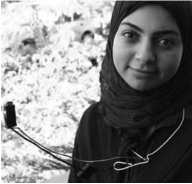
Above: Rana el Kaliouby wearing one of the Social-Emotional Wearables for autism spectrum disorders she designed, dubbed Head Cam . The device consists of a pen-sized camera, a small computer, and a wireless earbud that together provide the user with on-the-fly interpretations of facial expressions. The software evaluates the person's facial image and communicates its analysis by piping words into the user's ear, such as 'agreeing' or 'interested'. (Source: Rana el Kaliouby)
