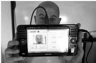
Above: Rana el Kaliouby, The Interactive Social Emotional Toolkit (iSet) designed to identify the emotions expressed in a person's face. To use it, one points it at a person much like one would point a camera. When the computer thinks it's identified a facial expression, a colored dot appears above the corresponding label. The dot grows larger as the computer becomes more confident it has identified the correct emotion. (Photo: Victoria Arocho for the Boston Globe)
