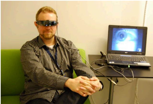
Figure 3. Screenshot from the video recording of a participant during test tasks. The eye of his pair is shown on the laptop screen and inside his near-eye display (NED) glasses.
