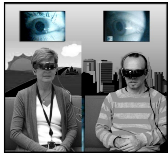
Figure 1. A pair sitting in separate spaces, using the eye-based video conferencing system. Each person sees a full-screen picture of the other person's right eye through the near-eye display. In addition, they can communicate through standard voice-over IP audio.
